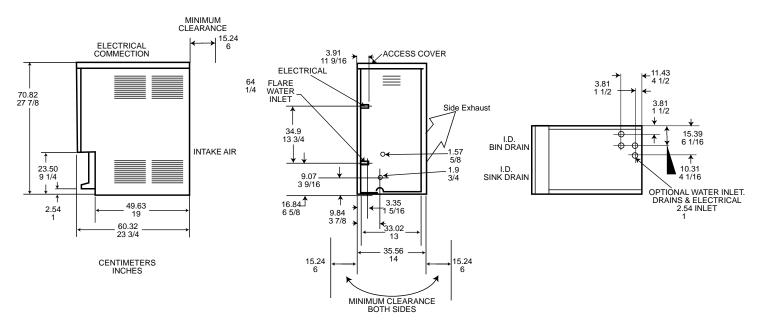
INSTALLATION NOTE: Allow 6" minimum space at sides and back for ventilation and utility connections.
